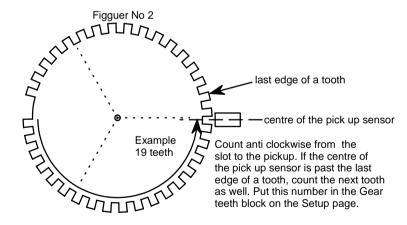
In this example the slot is past a third of the gear. This means that the ECU will fire on coil 3 first, then on coil 1 and then on coil 2. This setting will be 19 teeth - 12 teeth = 7 teeth and then about 6 degrees for the BTDC setting. For a 60-2 gear the subtract value is 20 instead of 12.
