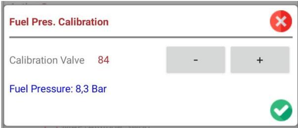
If you have an accurate fuel pressure gauge or a different fuel pressure sensor you may calibrate it with this value. It is a percentage correction which allows for range calibration only. That means calibration is accurate at the working pressure. The sensors supplied are calibrated according to the manufacturer signal specs. See the **Fuel Pressure Sensor Settings** page for other adjustments.
