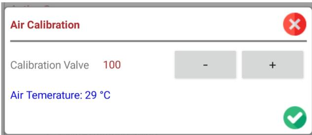
Reduce or increase the value to slightly shift the reading value. Do this at the critical temperature for instance where the engine is at running temperature. If the error is large you may need to replace it or get the correct sensor.
