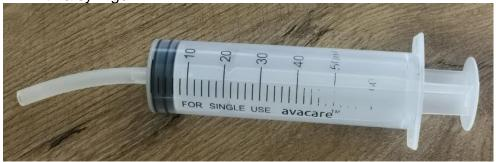
This method gives best results fast. Especially if you have the specifications of the sensor. You will need a 50cc Syringe and a short 3mm hole silicone rubber pipe. Look at the specks of the sensor. Below is an example:
