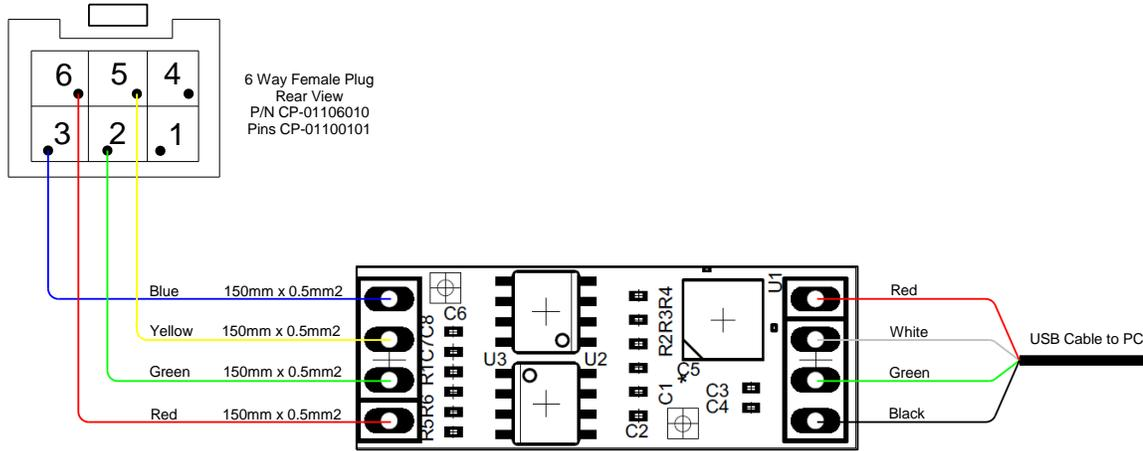
This connection diagram indicates where the wires is connected encase a cable gets damaged.
