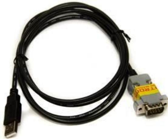
The Prolific RS232 to USB converters were popular in the old days and could be used only for TCU, EMU and Titan units. Note however that you had to break-out pins 1, 4, 6, 7, 8 & 9. This is due to other connections from the ECU to the 9 pin D-sub connector. Use a small screwdriver and bend them outwards and then inwards till they break out. Do not damage the other pins. There are small numbers inside. Below is an illustration of the layout.
