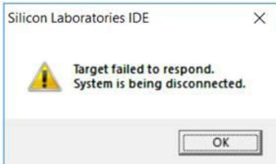
This message appears when the debug adapter makes only partial connection to the device. Usually a damaged Micro Processor of the device.
