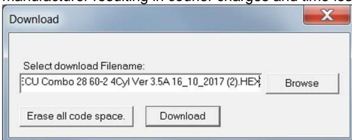
Disconnect all the output harnesses from the product. The programmer will switch the outputs to the high state which means that coils and injectors will be switched on. This may damage the coil drivers or coils and fill the engine with fuel.
