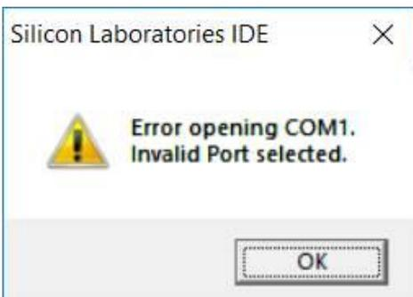
This message appears when the debug adapter Connection Options settings is incorrect. See the example below.
