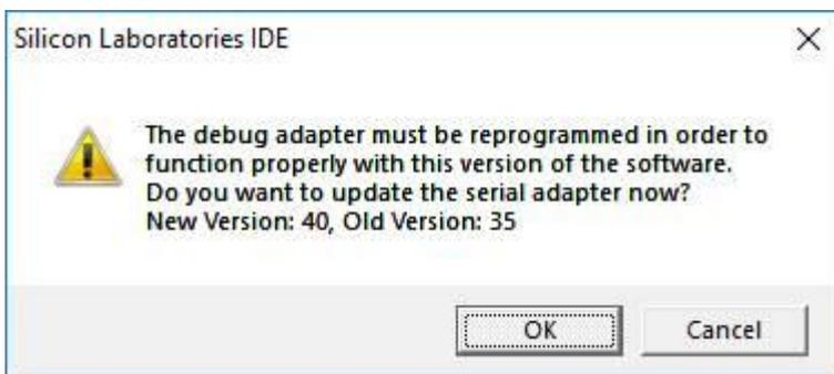
This message appears when the Silicon Laboratories IDE Software and the debug adapter are not the same version. If you press Ok it will be updated and never ask this question again until you load newer version Silicon Laboratories IDE software on the laptop.
