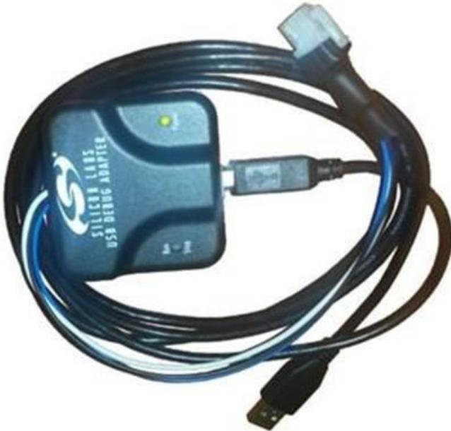
The USB Debug Adapter or Firmware Programmer as we call it in the manual, are used to download updated firmware or other firmware into the devices. This unit requires software to be installed and can be downloaded from [www.spitronics.com](http://www.spitronics.com). You may click on the bottom link to download the software.
