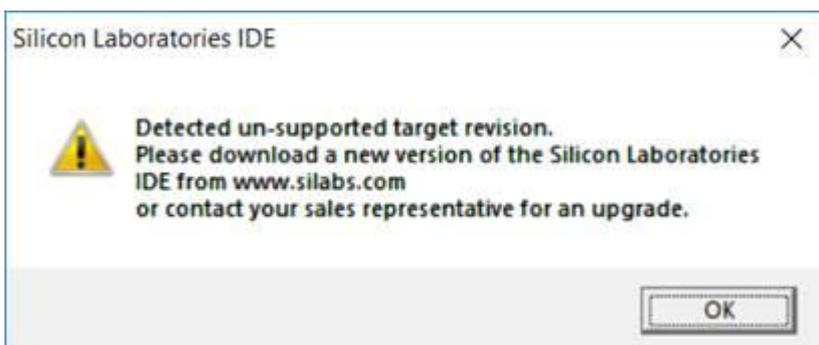
This message appears when the debug adapter is not connected to a Spitrionics device. It may be a broken wire between the debug adapter and device. It may also be a faulty device. Usually when the Micro Processor of the device is blown. It may also be a damaged USB debug adapter. On some products the
