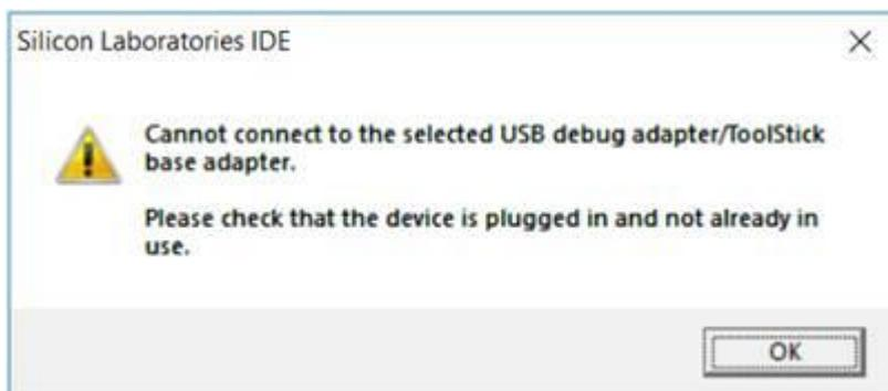
This message appears if the debug adapter is not connected to the laptop. If it connects the Run and power LED's will light up on the debug adapter. It may also be a faulty debug adapter.
