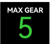
This value displays the highest gear that the TCU may select. This is a driver selection to prevent the TCU from selecting higher gears.
