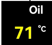
This value displays the current TCU oil temperature if the box has a sensor.
