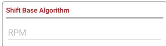
This block is for future use on specific firmware. Current firmware can only base calculations for profiles on the RPM signal with Speed limits implemented. In future firmware will be developed for speed base calculations.
