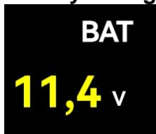
This value displays the current battery volts measured at the TCU.
