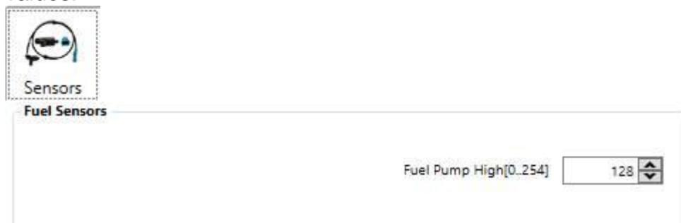
Now go to the fuel pages and set the ACC values to Zero. This represents opening and closing PWM or Duty Signals and then Gain or Proportional settings.
