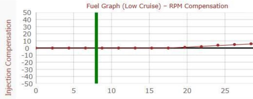
Now when the engine hunts we will use timing to control it before the idle valve needs to act. First you must understand what happens in hunting. The engine will lose power resulting in an increase in manifold vacuum. The vacuum bar will move to the right and the RPM bar will move to the left. Due to our slower timing we can increase timing to add power which will increase RPM. Adjust the Low rpm timing graph as below.
