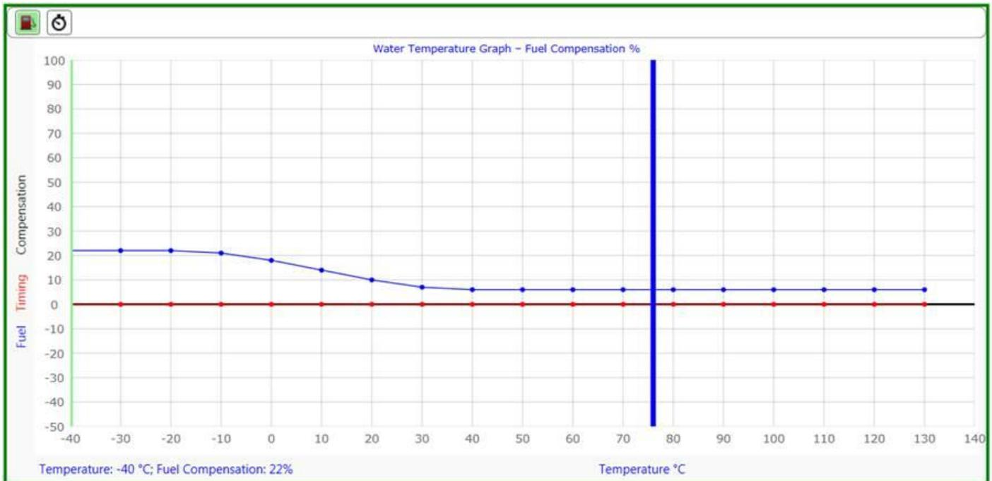
If the Water Temperature setting is off, then there will be no water temperature compensation for cold start. The Idle Control Low Limit Duty Cycle value will be used as idle setting.
