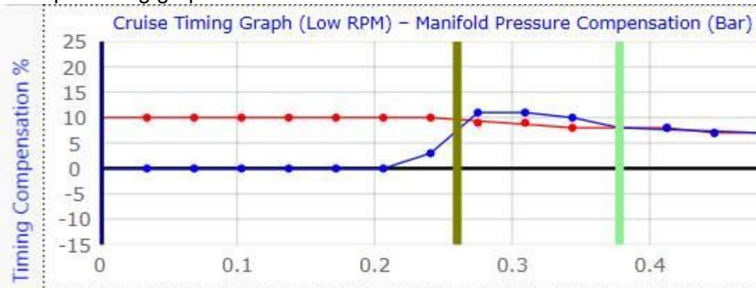
Lower rpm also brings more air in the manifold which requires a bit more fuel to make the mixture a power mix. Adjust the green and brown graph on the RPM graph as the lower rpm range to add a certain % fuel. Note on the fuel load graph we already should have a slight increase in fuel.
