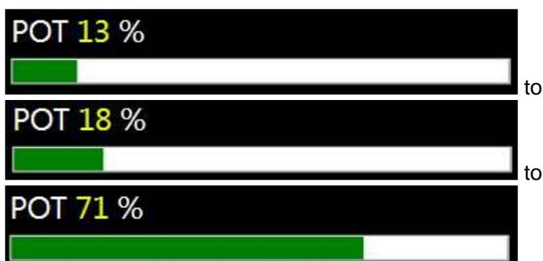
Also note if the action is inverted. It must be rising in value with increase of throttle. If it is falling volts with opening, then it may be incorrect connection of the 5 volt and ground wires.
