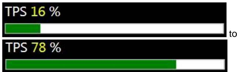
Also note if the action is inverted. This will help setup the pedal logic on rising- or falling edge later during calibration. The standard setup is rising volts with throttle depression. It may be an incorrect connection of the 5 volt and ground wires which may be swapped around. Below is the calibration tab when it is opened to indicate rising edge.
