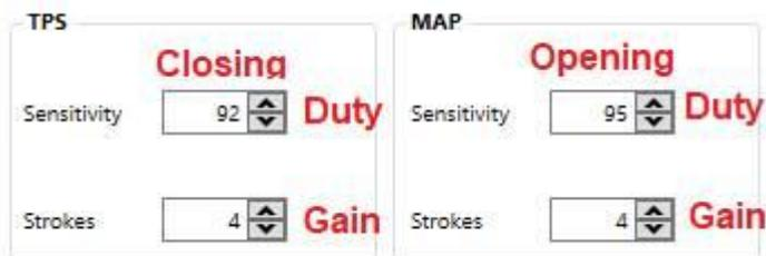
Now press the pedal slowly so that the throttle read the same as rest point. Take it slowly above the rest point and back. Notice if the throttle shudder excessively on the transition point. If it does vibrate or seem to have a dead band, increase or decrease the Map Teeth and see where the throttle is smooth when it passes the rest point with the least amount of shutter. Save the settings to the device.
