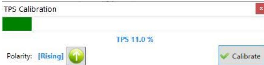
Calibration is done by stepping on the pedal and releasing it. The min and max values will be populated in two positions in the calibration window.
