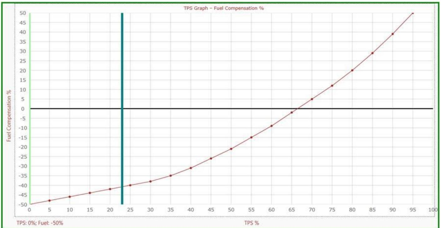
After setting, make sure the throttle can move over the whole scale range. Note that *Low Limit Duty Cycle* will cause the throttle to not go to 0% but remain it idle %. You may start the graph at a higher value than -50% so that the throttle moves more instantly when the pedal is pressed. Make sure not to set it too high, as it will then overcome the min duty cycle and the engine will idle faster.
