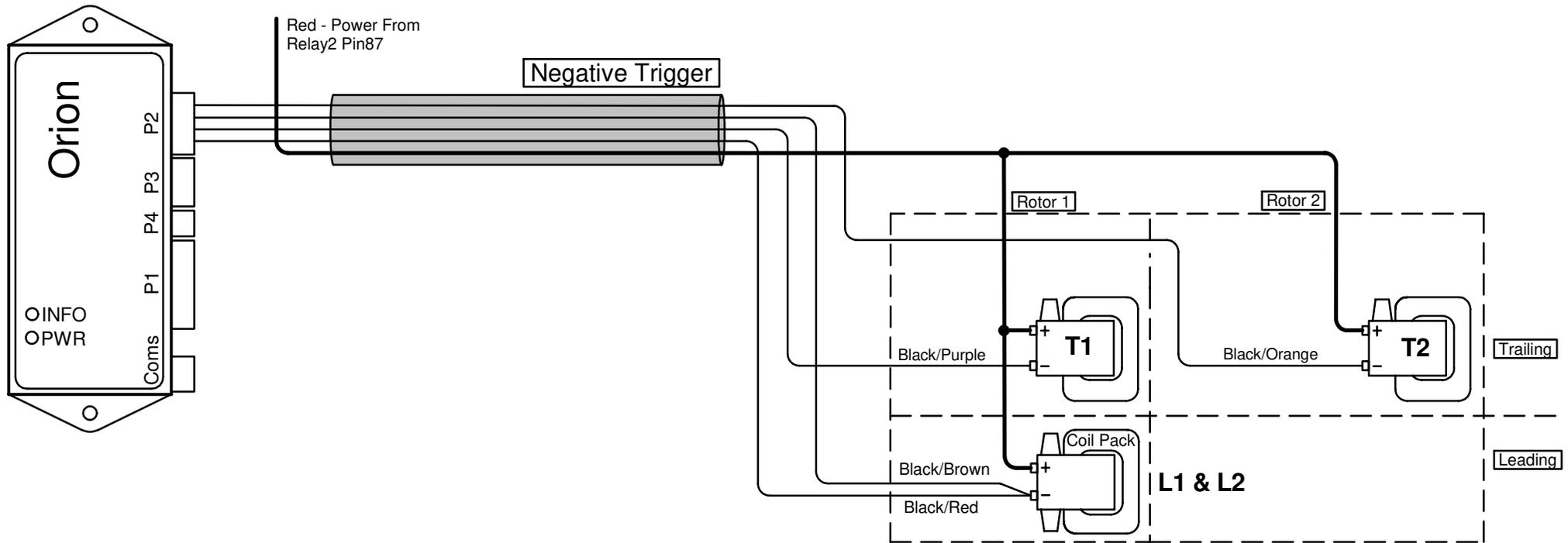
**Note:** The 2 leading coil drivers are tied together on the wasted spark leading coil pack. Software must be set to wasted spark. The trailing coils cannot be shared with a coil pack.
