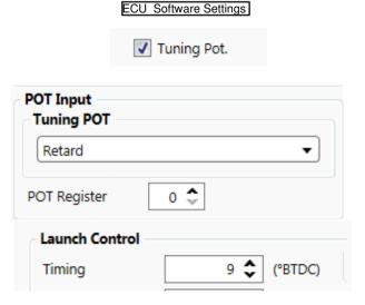
**Note:** The connection from the Orion TCU changes with its GP Output Priority selection. View the Priority spreadsheet for the specific firmware to see which output is used as Retard output. It will be a negative driver.
