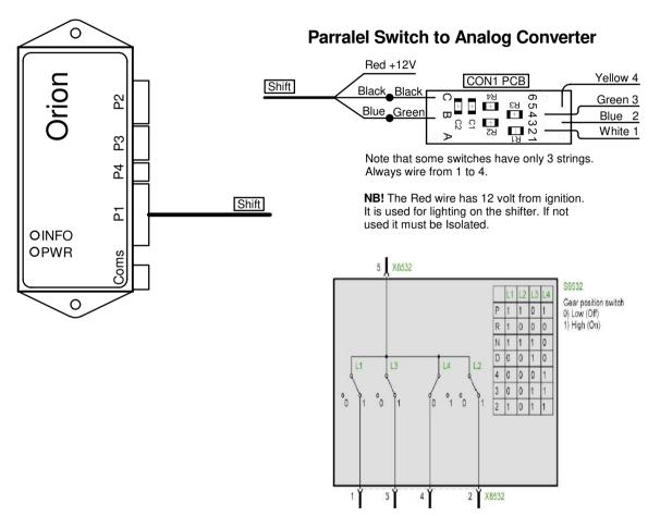
Example of a parallel switch. One common wire will switch to multiple position in paralel creating a binary code combination.
