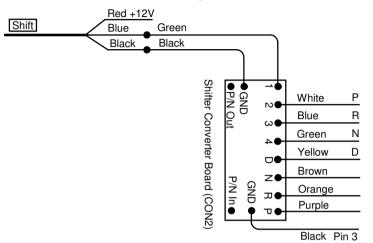
Note that the shifter positions on the board is incorect. Always use the wire side position numbers.
