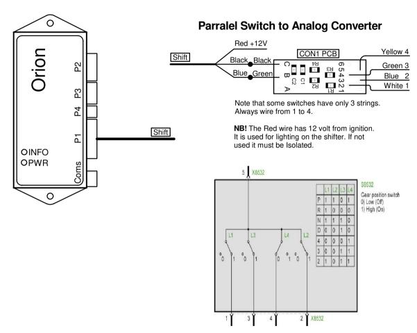
Example of a parallel switch. One common wire will switch to multiple position in paralel creating a binary code combination.
