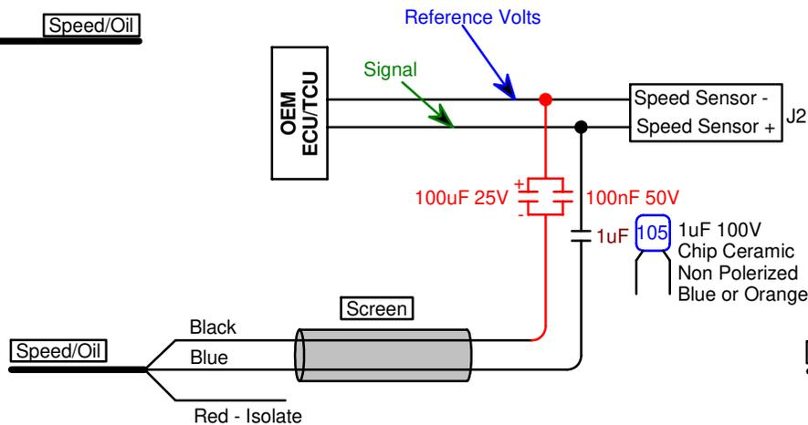
Note! Optional Capacitors from reference to black will help prevent interference in ECU earth differences
