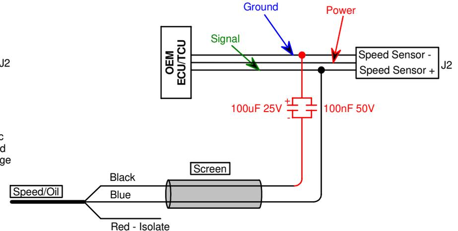
Note! Optional Capacitors from reference to black will help prevent interference in ECU earth differences
