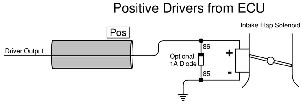
**Note:** The connection to the Mercury ECU changes with the GP Output Priority selection, View the Priority spreadsheet for the specific firmware to see which output is selected. Then make sure on how to connect between the 2 options above. It could be connected on a negative or positive driver.
