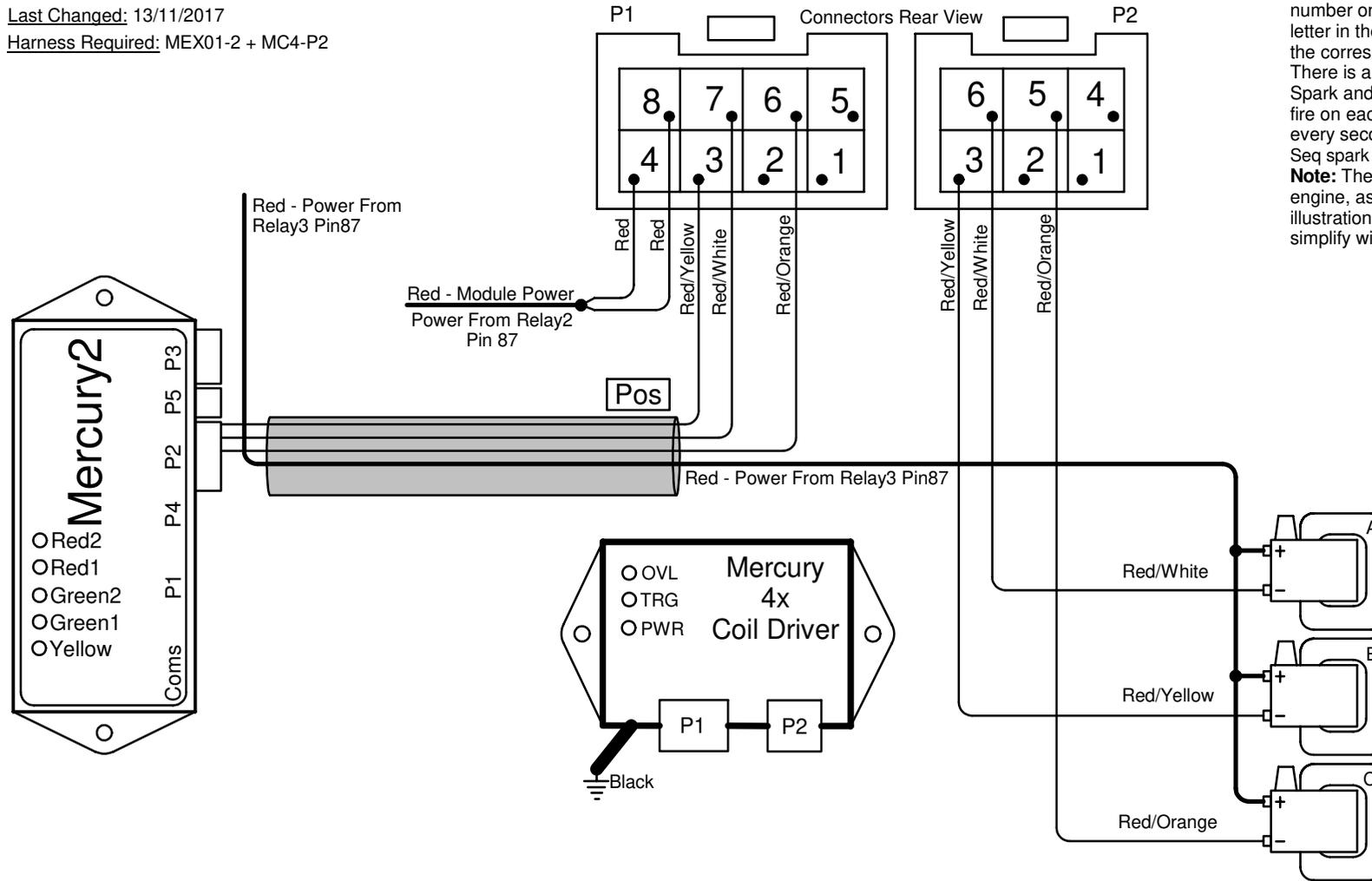
Write your firing order from left to right in the blocks above marked with an alphabetical letter. Then write the corresponding number on the corresponding coil with the same alphabetical letter in the drawing below. Now connect your coil number to the corresponding color wire.
