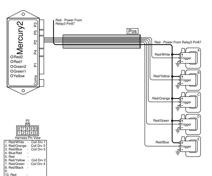
Write your firing order from left to right in the blocks above marked with an alphabetical letter. Then write the corresponding number on the corresponding coil with the same alphabetical letter in the drawing below. Now connect your coil number to the corresponding color wire.
