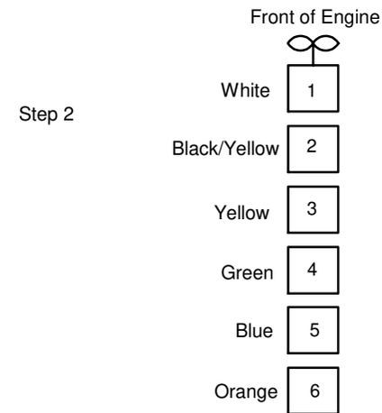
Write the corresponding colour of each cylinder next to your injector number on the lines marked X on the drawing. This will ensure that the sequence of injection is correct.
