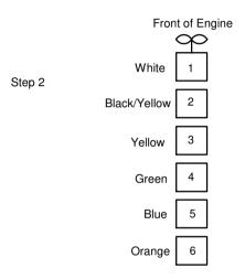
Write the corresponding colour of each cylinder next to your injector number on the lines marked X on the drawing. This will ensure that the sequence of injection is correct.
