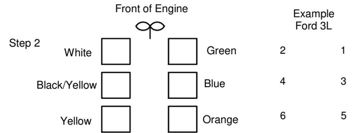
Write the cylinder layout of your engine in the blocks above. Make sure which side is the No1 cylinder and how they are numbered on your engine. Then write the corresponding colour of each cylinder next to your injector number on the lines marked X on the drawing. This will ensure that the sequence of injection is correct.
