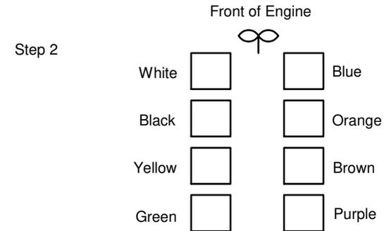
Write the cylinder layout of your engine in the blocks above. Make sure which side is the No1 cylinder and how they are numbered on your engine. Then write the corresponding colour of each cylinder next to your injector number on the lines marked X on the drawing. This will ensure that the sequence of injection is correct.
