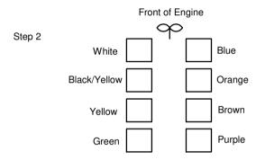
Write the cylinder layout of your engine in the blocks above. Make sure which side is the No1 cylinder and how they are numbered on your engine. Then write the corresponding colour of each cylinder next to your coil number on the lines marked X on the drawing. This will ensure that the sequence of spark is correct.
