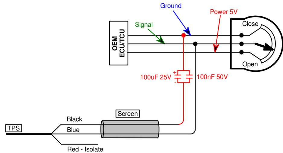
Note! Optional Capacitors from reference to black will help prevent interference in ECU earth differences
