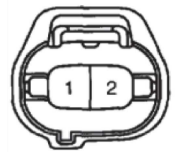
Transmission Selector Switch NB! Transmission Plug Pin View
